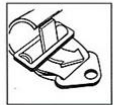
Step 4: Fold back webbing again and insert through bottom of 3-bar slide.
